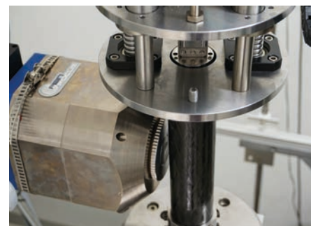
The specimen assembly is pushed into the CFRP tube from above.
